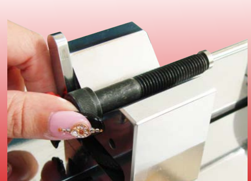
Thread length measuring
